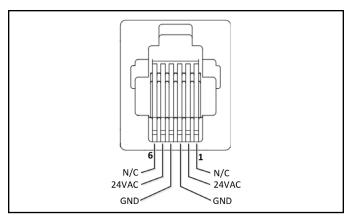
Figure 8. Pin-out of the console's power socket
